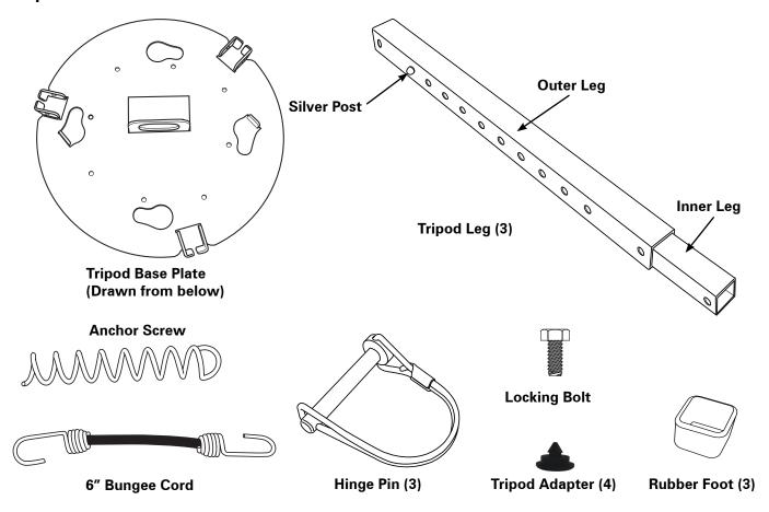
The Carryout Tripod is designed only for use with portable satellite TV systems. The tripod has a maximum supported weight of 20 lbs. DO NOT use the tripod as a step or a seat.
